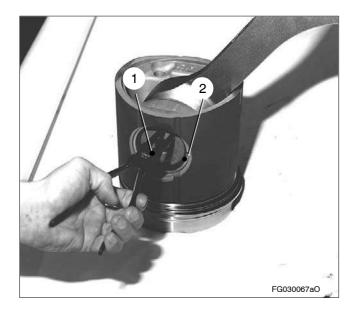
Insert second snap ring (2) with snap ring pliers (1).
