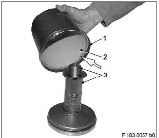
Insert new insert sleeve (2) into rotor hood (1).
