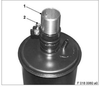
Insert sleeve (1) and tighten with hex screw (2).
