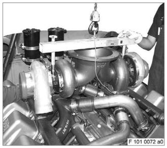
Unscrew hex nuts (1) on flange of exhaust turbocharger (2), left and right engine side.
