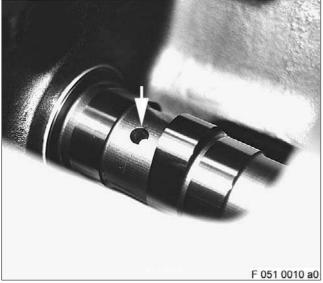
Locating bore (arrow) for locating device dowel pin.
