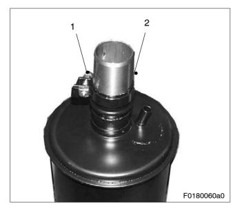
Unscrew hex screw (1), withdraw sleeve (2) from oil separator and remove.
