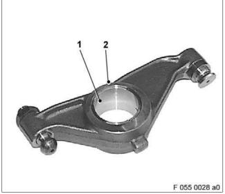
Insert adjusting screw (2) into valve bridge (1). Attach nut (3) to adjusting screw; do not tighten!
