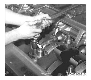
Measure shaft length of conrod screws; for max. shaft length – see C 037.05.01.
