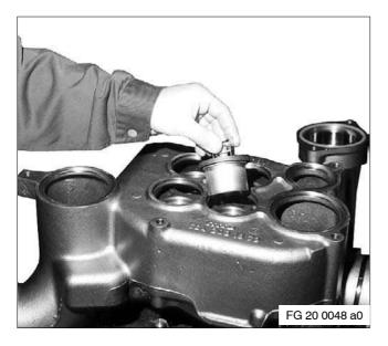
Removing coolant distribution housing
