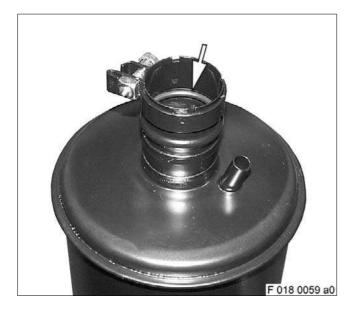
Coat O-ring (arrow) with denaturated ethanol. Insert sleeve, see next illustration.
