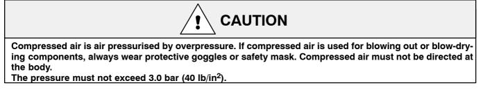
Blow out oil lines with compressed air and ensure that they are, perfectly clean.
