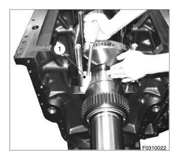
Position jig (1) between bearing cap stud and rear face of shell on side where butting joint is.
