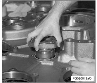
Mark axle according to installation position and remove from equipment carrier.
