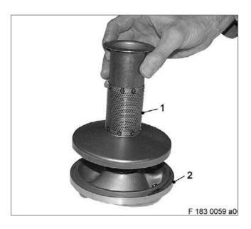
Remove standpipe (1) from rotor substructure (2).
