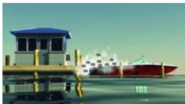
Blockage of boat exhausts by obstruction.
