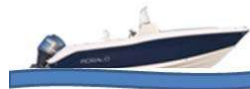
Incorrect Causes boat to "porpoise"
