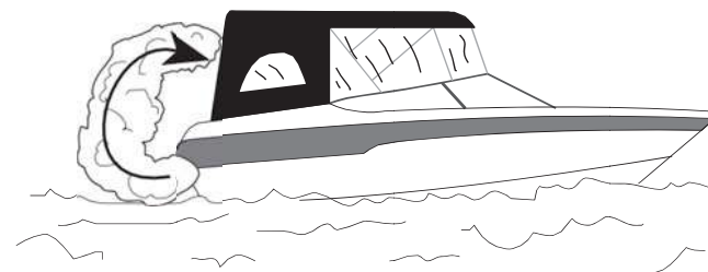
Figure 2.3 - Exhaust accumulations while canvas is in place
