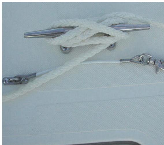
**Anchor Line Secured to Cleat**
