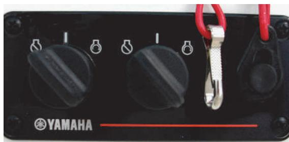
**Engine Stop Switch Lanyard (Typical)**
