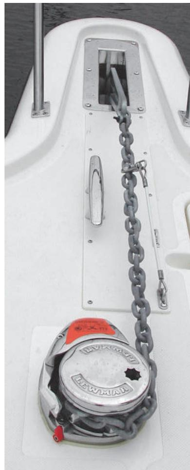
**Anchor Chain Properly Secured for Travel**
