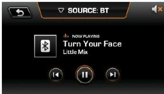
Like the Audio function within the PV1100, the PV450 allows the various sources to appear. Touch the Source area and choose between AM/FM Radio, Bluetooth, USB, NOAA and Aux.
