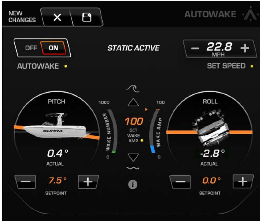
AutoWake\* is a patented system that will manipulate the ballast levels in order to achieve and maintain the best possible wake for surfing and wakeboarding. Using an inclinometer (a device that measures angle of pitch and roll) the boat will orient itself for the best boating experience.
