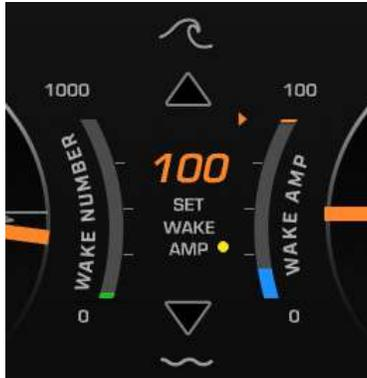
Use this setting to define the amplitude of your wake (0 is mellow and 100 is aggressive). The Wake Amp\* bar will fill (in blue) or empty to the target Wake Amp setting (orange pointer). This blue fill will indicate your total fill level for all ballast.
