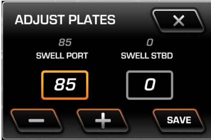
Utilize the – and + keys to adjust the chosen plate. Touch Save when done, or X to exit without saving the changes.
